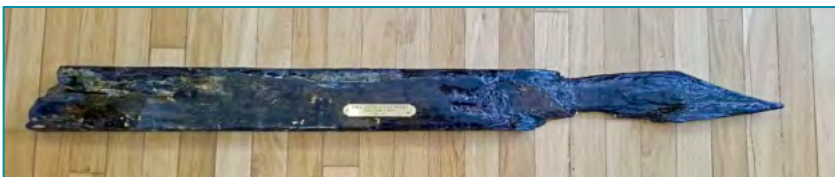
Philo Farms center point survey post, made from pine heartwood. Placed in 1912 and removed in 1977 by surveyor Dan Dailey. Donated to LRHS by Gary Garrison.
